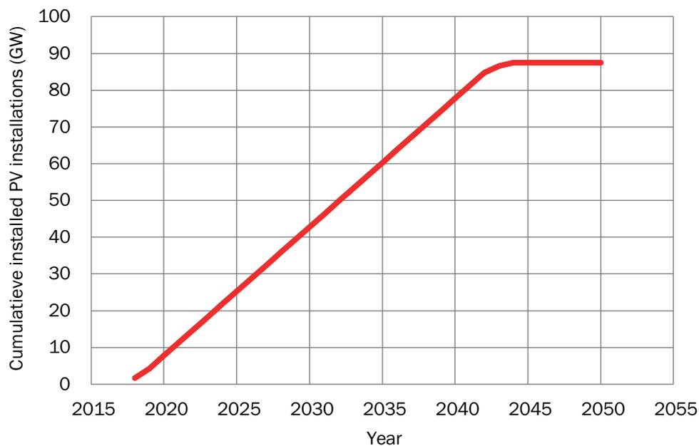
Figure 1. Growth curve based on 3,5 GW of PV installed per year from 2020 onwards and 25 year product lifetime
