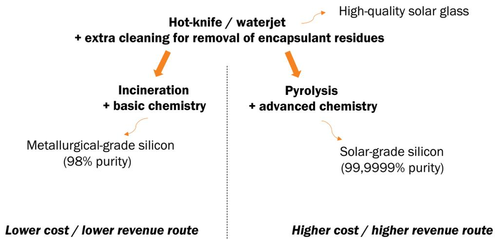
Figure 4. Recycling routes incineration and pyrolysis
