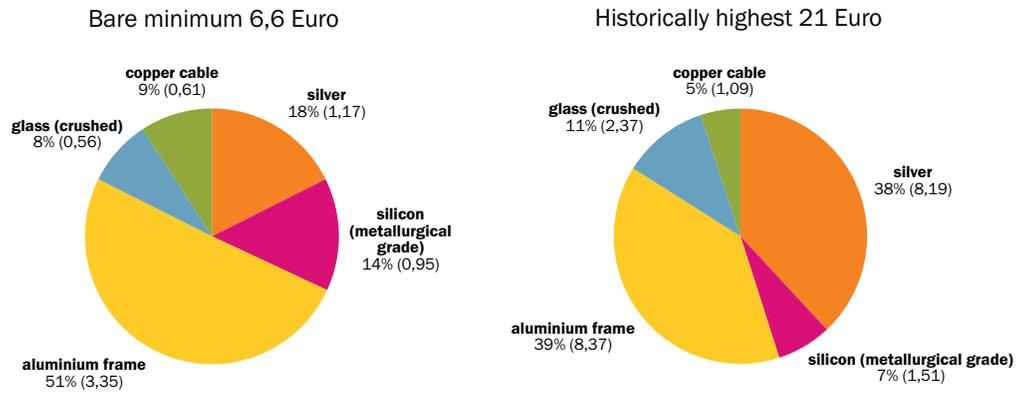
Figure 6. Minimum and maximum revenue for all valuable materials extracted, assuming metallurgical grade Si and crushed glass. Absolute material values in euro are given in brackets.
