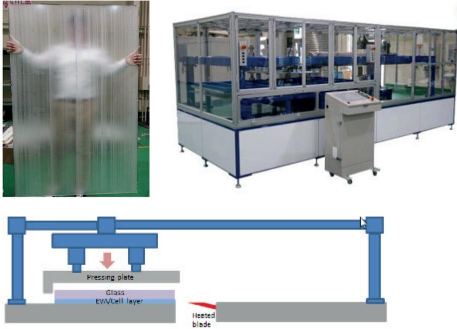
Figure 9. Left, PV glass plate after separation with polymer residue. Right, NPC Japan hot knife glass separator installation. Below working principle of the hot knife installation
