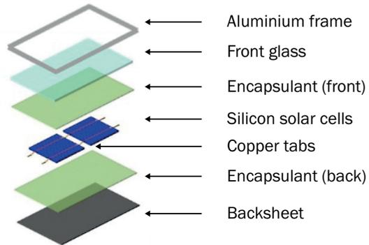
Figure 7. Cross section of a contemporary standard PV panel
