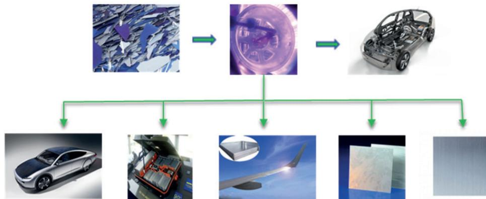
Figure 13. Silicon solar cell waste, physical process, lower grade 99,6% purity for low weight high strength materials and e-car battery silicon-anodes. Final goal production of new solar cells with solar grade (9N) silicon
